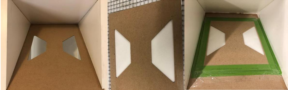
**Figure 1: (Left) Permanent mounts were sealed in place and allowed to cure prior to use. (Middle) Test materials were mounted on the back of the filter holder along the seams. (Right) The mask was aligned and held in place with painter’s tape, followed by 2 layers of heavy-duty packing tape to seal the edges.**
