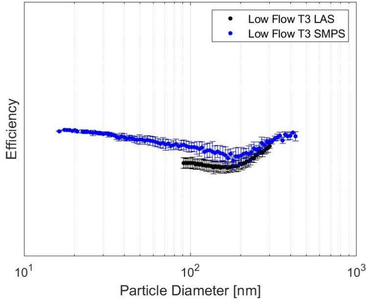
**Figure 5: The performance of the Material #4 sample during SMPS testing outperformed the average efficiencies of the LAS measurements. This anomaly in results may be attributable to a variation in the singular Material #4 sample tested with an SMPS. Additional test articles of this material have not been tested with an SMPS so the source of this discrepancy has not been determined.**
