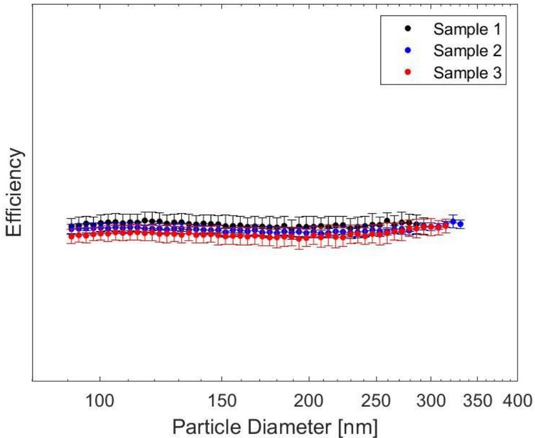
**Figure 3: Sample 1 was a pristine N95 respirator sample that received minimal handling prior to testing. Sample 2 was used for a fit test by one individual prior to testing. Sample 3 was a clean control sample but the amount of handling and method of storage prior to testing was not known.**
