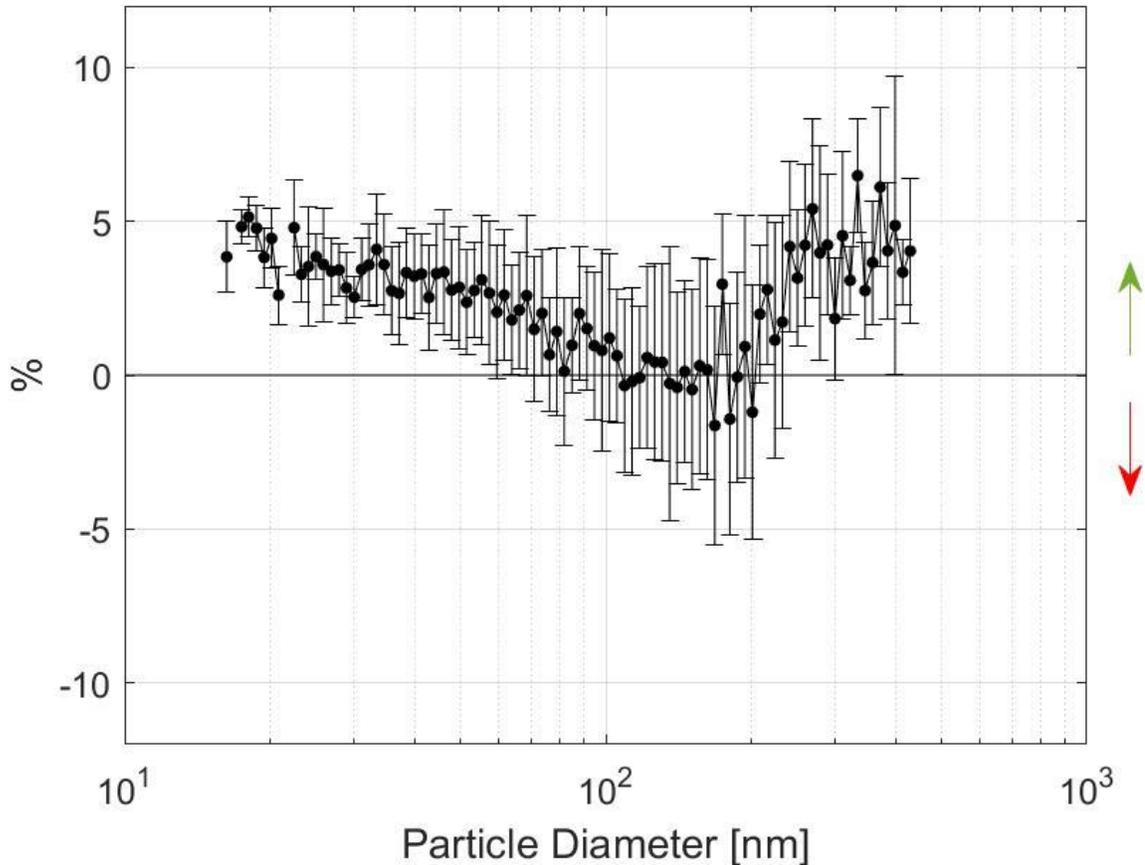
**Figure 7: Comparison of efficiency results between Material #4 and Sample 2 using SMPS data. The SMPS was able to provide statistically significant data at smaller and larger particle sizes than the LAS.**
