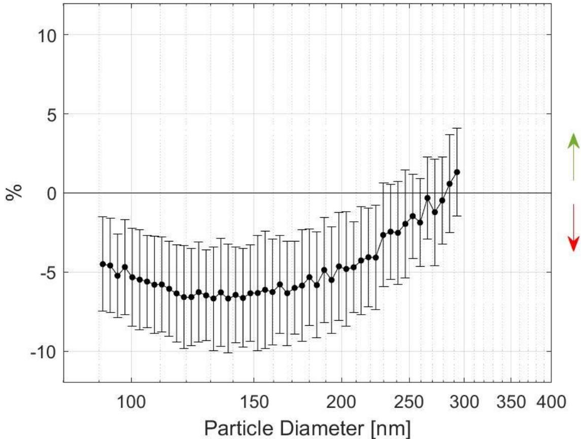
**Figure 4: The difference in efficiencies between Material #4 versus the N95 control was plotted as a function of particle size ( $E_{M4} - E_{N95}$ ). The lower-half of the graph (red-arrow) indicate where Material #4 underperformed and the upper-half (green-arrow) indicates where better performance was observed from Material #4.**
