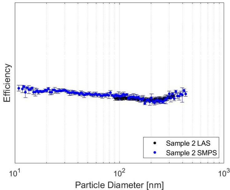
**Figure 6: Testing of the N95 mask, Sample 2 from Figure 3, at low flow with both instruments yielded results with strong correlation. No filter loading was observed. The presence of filter loading would be signaled by a noticeable increase in the pressure drop and efficiencies over the course of subsequent measurements, neither occurred.**
